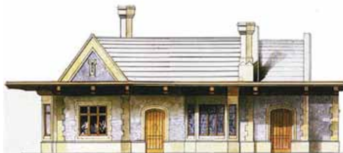
The station was built to the most elaborate of Brunel's standard designs, and constructed from Bath stone
